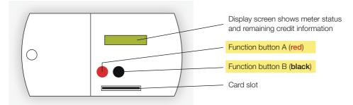
This meter is operated by a Quantum Card. To function properly this card must be registered with the meter. Cards can only be obtained from your gas supplier.
